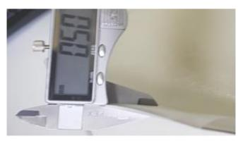
Fig. 3. Thickness measurement of paper in a sleeve, which determines the distance between each pair of tags.
